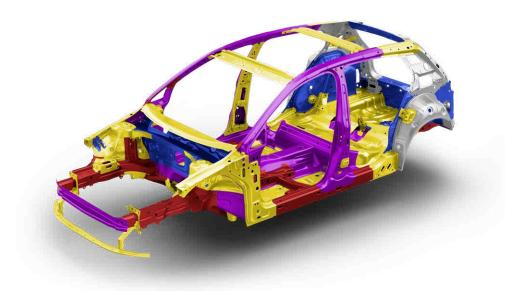
The structure of the all-new Golf R-Line is built with a combination of 5 steel types that increase rigidity and provide optimal safety. At the same time, its structure remains lean and sturdy, so that the overall vehicle is light and carries itself effortlessly. The result? You'll feel a more agile, precise, and efficient driving experience.
